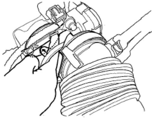
Fig. 29: Pushing Throttle Valve Closed Courtesy of AMERICAN HONDA MOTOR CO., INC.
